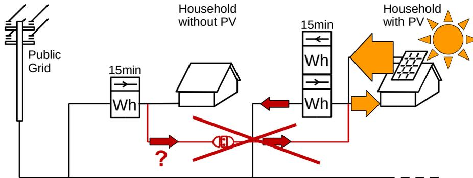
**Fig. 2.** Energy sharing with a power cord. Take care: This leads to uncontrollable current flow!
