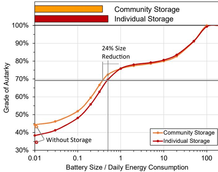
**Fig. 6.** Grade of autarky for the settlement with a community storage compared to average grade of autarky of the households with individual battery storages. Both storages have the same accumulated capacity.
