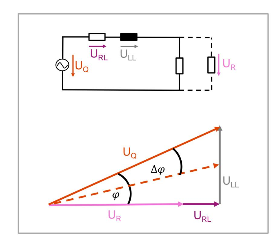
A pointer diagram can be made of the values of the amplitude and phasor-angle. This is more precise than analyzing only the grid impedance, because the inductive share is located only in the wire (simplified model). Its influence depends on the current flowing through the wire, which again is proportional to the wires load.
