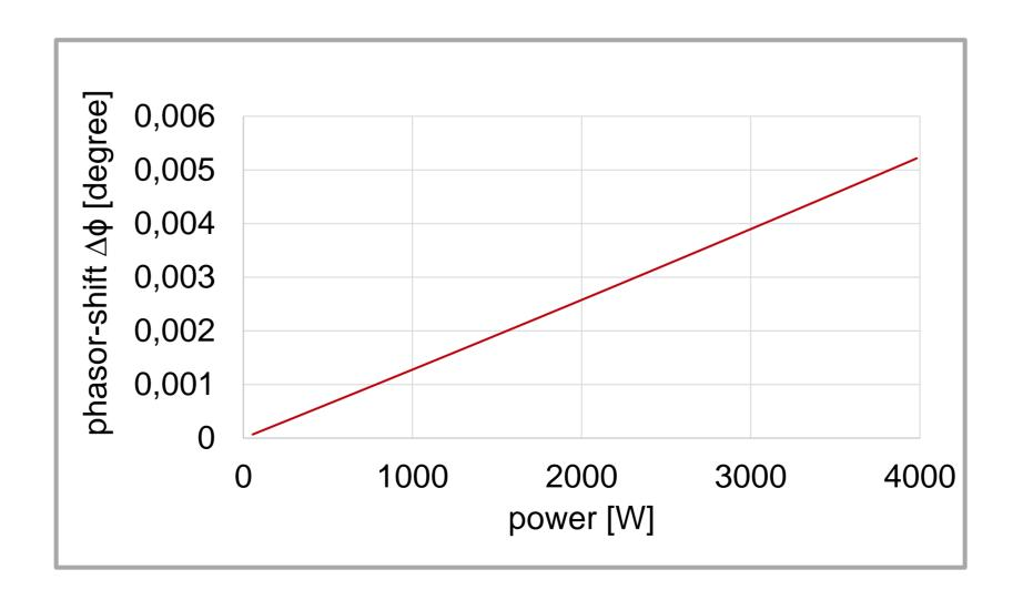
The phasor-shift related to the load power behaves linear. This was producible in simulations and measurements. From this, an exact determination of the load can be made. The phasor-shift appears with the same dependency for every string in the household. This is, because the inductivity of the cable to the house is a lot higher. No determination of the loads position can be done.
