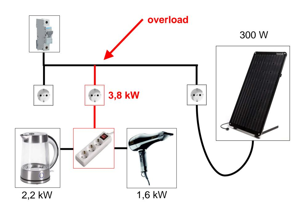
The fuse doesn't trip. No overload prevention is given. A PV-system has to detect this load situation and stop feeding.
