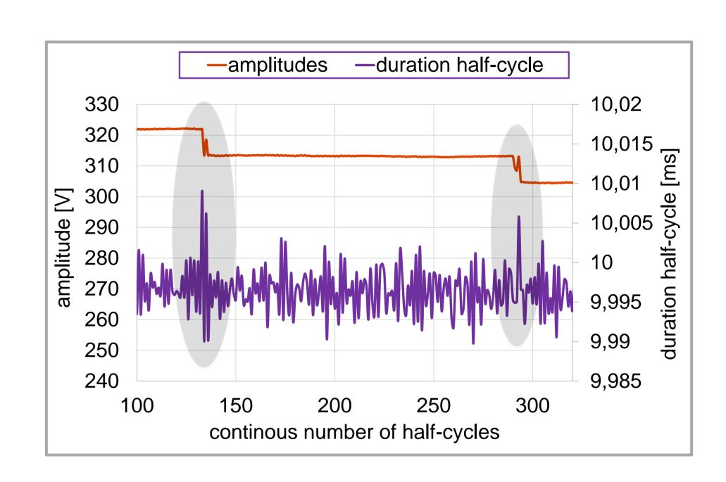
The duration of half-cycles in the grids sine has a natural variation, which is dimensioned in microseconds. The diagraph above shows, that load activations cause a delay of the same factor. Therefore it is difficult to estimate the load only by time delays. But still, some characteristics can be seen in the half-cycle durations. Fitting the values to a sine function and calculating the phasor-shift before an after load activation can help lowering the uncertainty.
