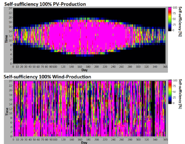
Figure 2: Self-sufficiency in form of a waterfall diagram, above a 100% generation by PV, below 100% generation by wind-power, created by a simulation
